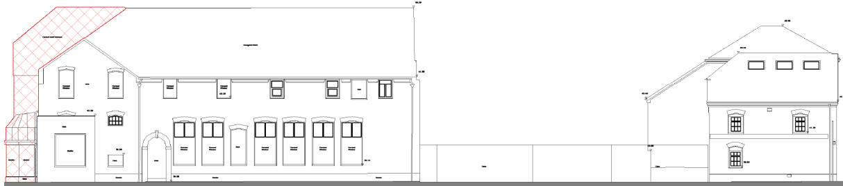
Northfield Road elevation - demolition shown in red
